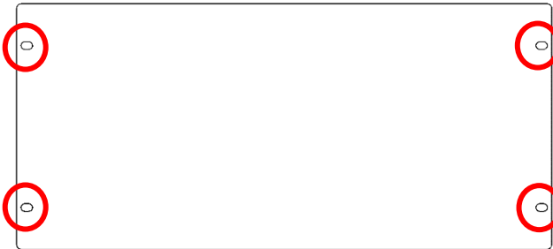
Figure 3a: 4x slotted mounting holes on front panel of units in measuring 1U - 5U in height.
